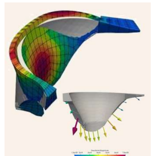
Study of the earthquake resistance of a dam with modelling of fluid-structure interaction and absorbing boundaries on the foundations.
