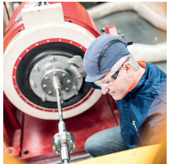
Vibratory pot simulating seismic loading
