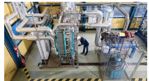
EDF R&D's high temperature heat pump lab allowing for testing of heat pumps up to 1MW and 150°C. © Lutt Julien, CAPA Pictures
